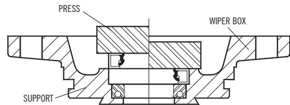
The mechanical seal contains a garter spring. Check to see that this spring is still properly located and in its position. The mechanical seal has a metal case which serves to force the Poly Pak seal into its cavity, energizing its lips. Apply oil lightly to the bore of the box before pressing each seal into its counterbore.
