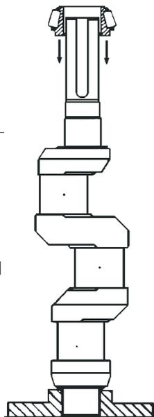
shimming is correct, the shaft will move laterally from .005" to .010".
