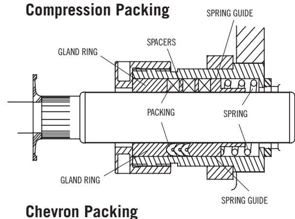
Note that the gland is screwed tightly onto the box and contacts its face. The spring is providing all of the initial compression and adjustment. No adjustment is provided by the gland.
