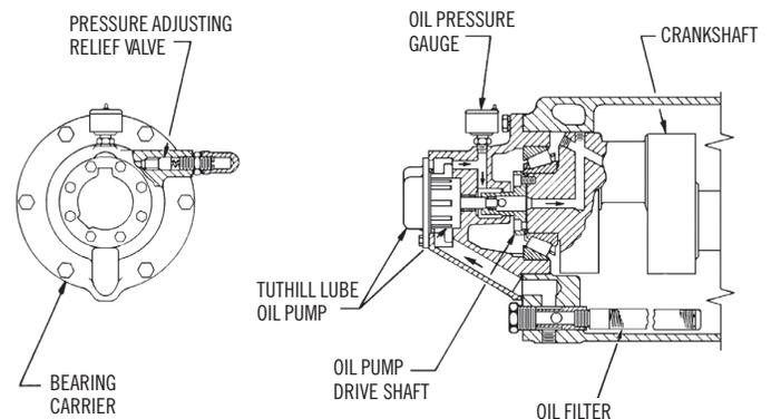
Lube oil pump and filter assemblies are employed in certain Myers Apex Series pumps. This assembly is installed after the shaft and its tapered bearings have been correctly set. Providing filtered oil under pressure (35 to 75 psi) to all crosshead pin bushings and crankpin bearings, this special gear pump is driven by a bloted-on drive shaft. Driver is made with a female drive square which drives the male square end of the lube oil pump shaft.
