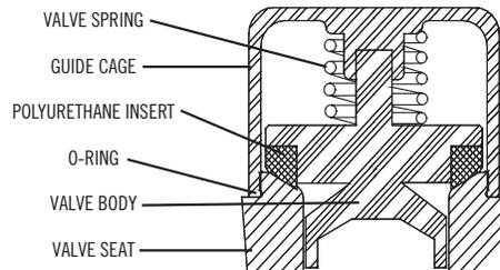
The Myers Apex Series valve is a precision made subassembly using threads cut into the rim of seat for use with Myers Apex Series setting/pulling tool. These threads do NOT deteriorate as proved by field experience. By locating these on the rim, setting/pulling forces are now applied only to the rim of the seat, never to the webs (or “spokes”), or to the center section. Distortion of the seat is eliminated.
