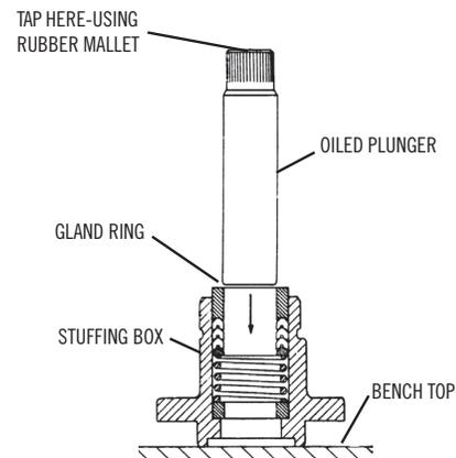
Apply oil liberally to plunger O.D. and lightly tap it through the packing.
