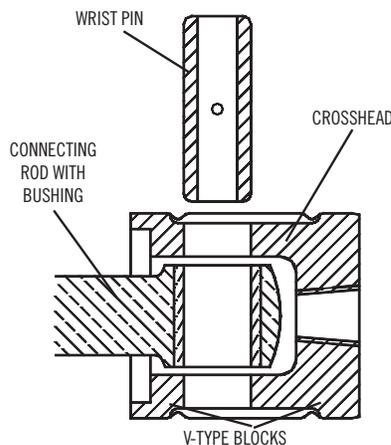
A mishap during insertion can occur causing the ruin of the pin or the crosshead, if during application of pressure:
