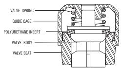
The Myers Aplex Series valve is a precision made subassembly using threads cut into the rim of seat for use with Myers Aplex Series setting/pulling tool. These threads **DO NOT** deteriorate as proved by field experience. By locating these on the rim, setting/pulling forces are now applied only to the rim of the seat, never to the webs (or "spokes"), or to the center section. Distortion of the seat is eliminated.
