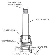
A soft rubber mallet is recommended to avoid any damage to the plunger face or its threads. Remember: The fragile nature of packing rings and plunger surfaces deserves your respect and avoidance of careless damage to these key elements!
