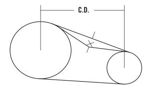
Sheaves must be balanced to prevent abnormal vibration. Balancing weights must **NOT** be removed. Type "QD" sheaves must be evenly tightened on their tapered hubs to avoid rim wobble and severe lateral vibration. V-belts that snap and jerk will produce abnormal vibration and loads on both pump and motor or engine.
