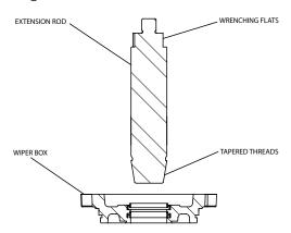
With extension rod inserted through the wiper box seal, thread the tapered threads (must be clean!) into the tapered crosshead female threads. Firmly tighten, apply torque to the wrenching flats only. Never damage the extension rod ground surface!
