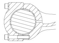
Check that all oil holes are clean and fully open. GRIT is the greatest enemy of bearings, however precisely manufactured. Hence, all surfaces must be perfectly clean and lightly oiled prior to assembly. Remove any burrs or sharp corners which prevent the perfect fitting of these precision bearings. Using a torque wrench, tighten cap bolts as follows:
