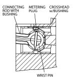
The hole in the wrist pin should line up with the hole in the connecting rod. Install the shoulder bolt through the wrist pin and thread into connecting rod. Torque to 25 ft.lb.
