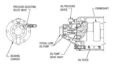
Lube oil pump and filter assemblies are employed in certain Myers Aplex Series pumps. This assembly is installed after the shaft and its tapered bearings have been correctly set. Providing filtered oil under pressure (35 to 75 psi) to all crosshead pin bushings and crankpin bearings, this special gear pump is driven by a bloted-on drive shaft. Driver is made with a female drive square which drives the male square end of the lube oil pump shaft.
