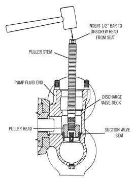
Effective pressure-sealing between tapered (male) seat and tapered (female) fluid end deck is possible **ONLY** if the tapers are absolutely clean and dry just prior to installation. Thoroughly clean surfaces using a clean solvent. Dry with a **CLEAN** shop towel.
