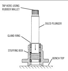
Apply oil liberally to plunger O.D. and lightly tap it through the packing.
