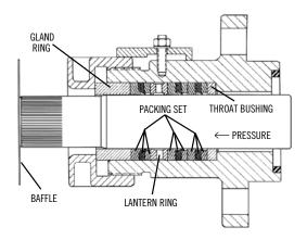
Above depicts Styles 838 and 858 packing correctly installed with all packing lips facing toward the fluid pressure. Note that two units of Styles 838 and 858 packing are positioned ahead of the lantern ring, and one unit is positioned behind it. Thus lubricant entering the lantern ring is forced toward the pressure.
